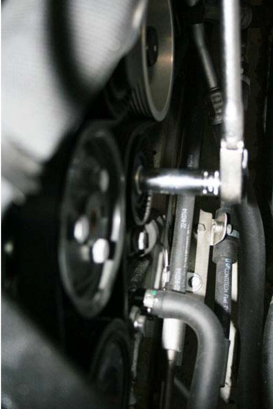
Remove IDLER pulley that is close to Water Pump pulley
