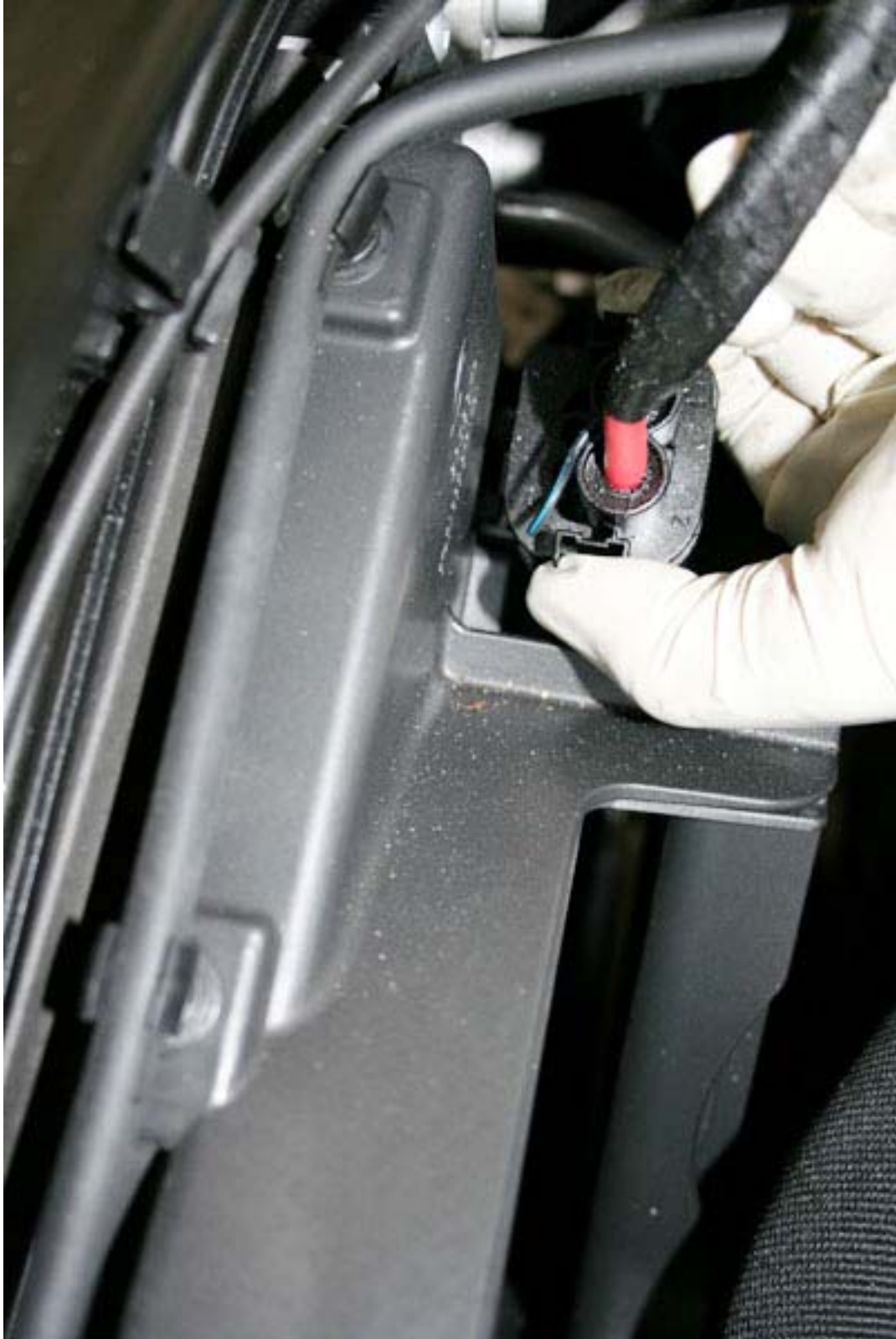
Disconnect engine aux fan connector
