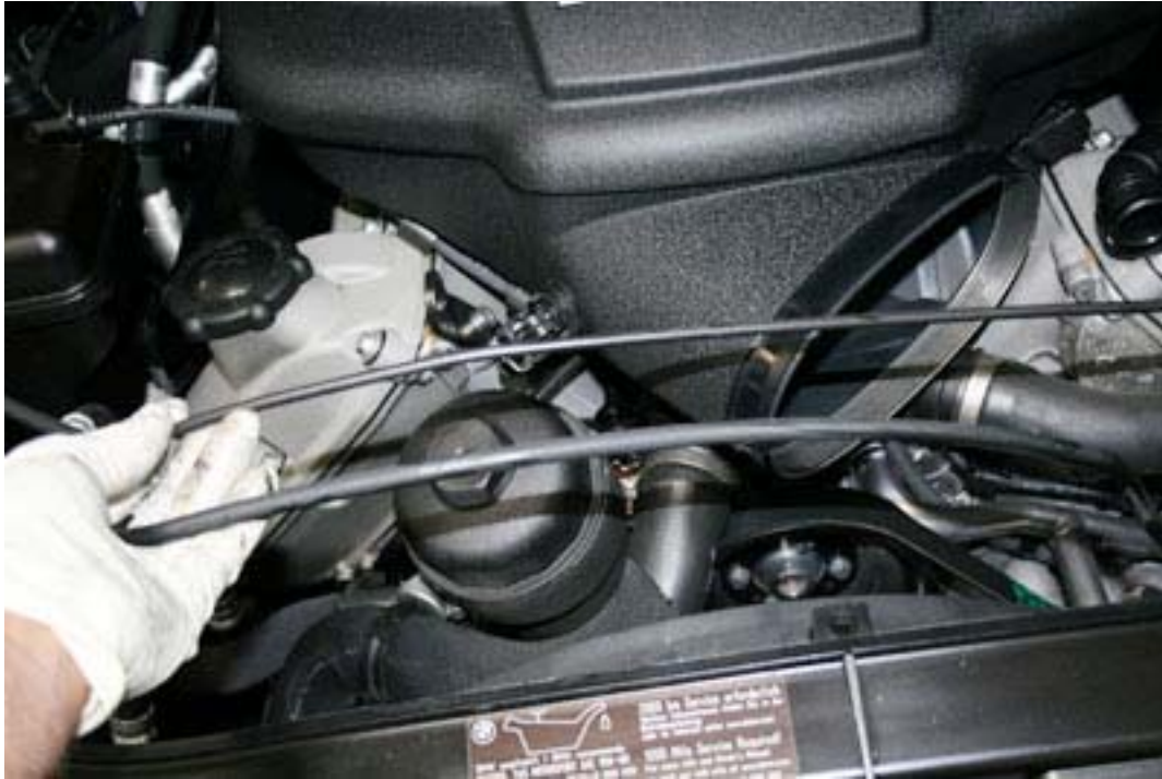
Move over flow hose and hood release cable away from engine aux fan shroud
