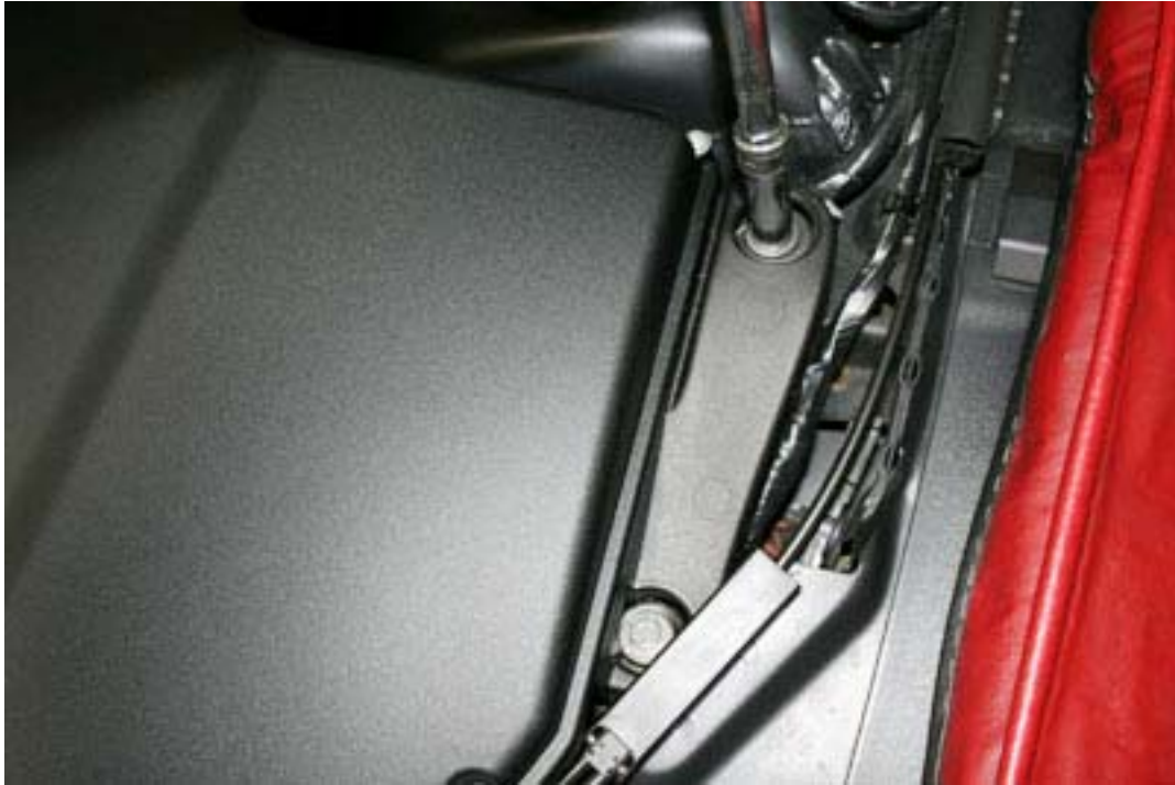
Unbolt using 10mm socket
