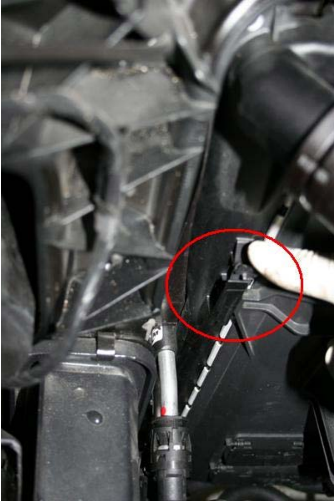
Release engine aux fan shroud clip on DRIVER's side to allow complete fan shroud removal
