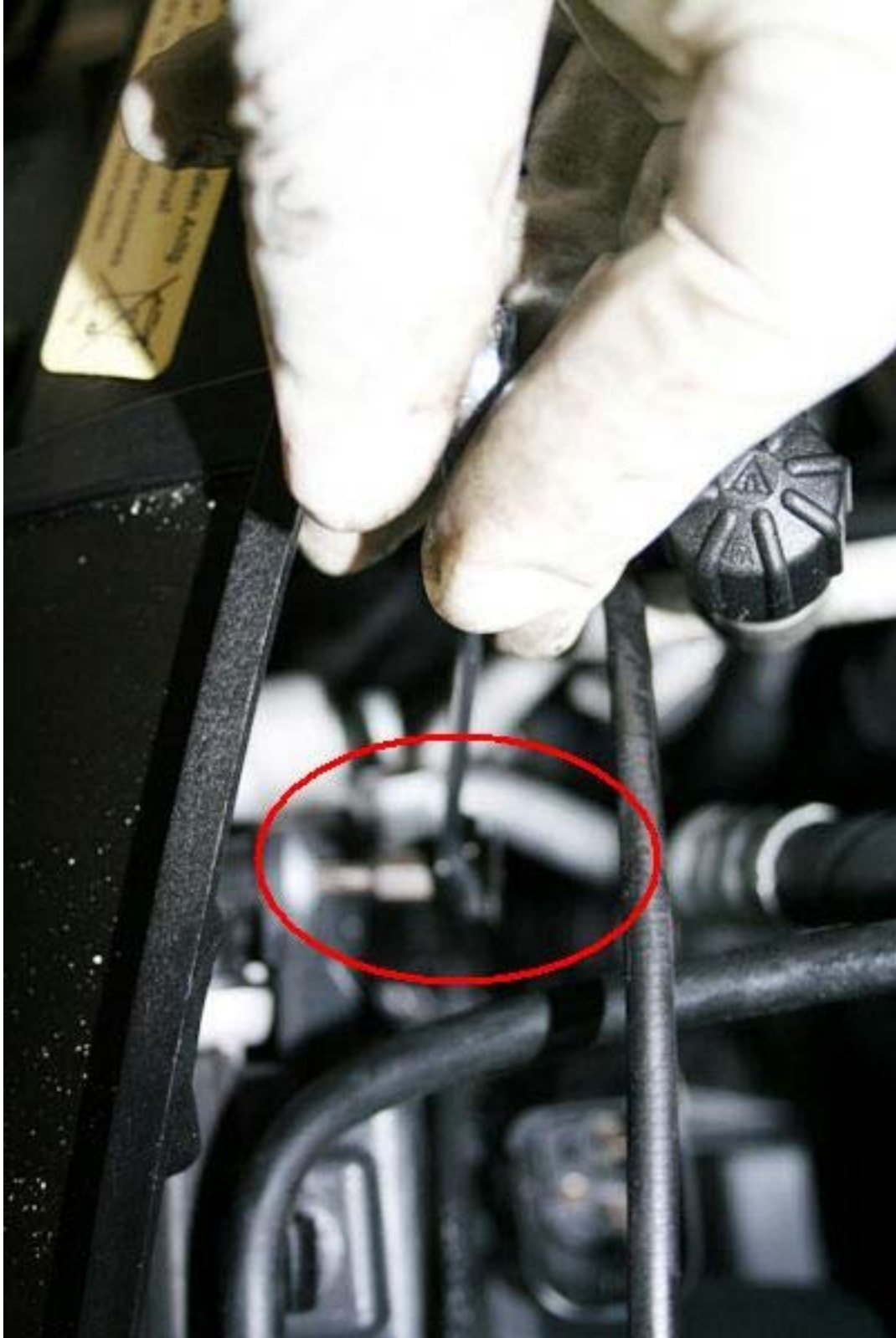
Remove bolt using Torx socket
