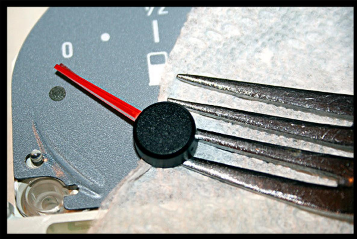
After prying the needles off, simply take the old gauge face off and slide the new one on.
