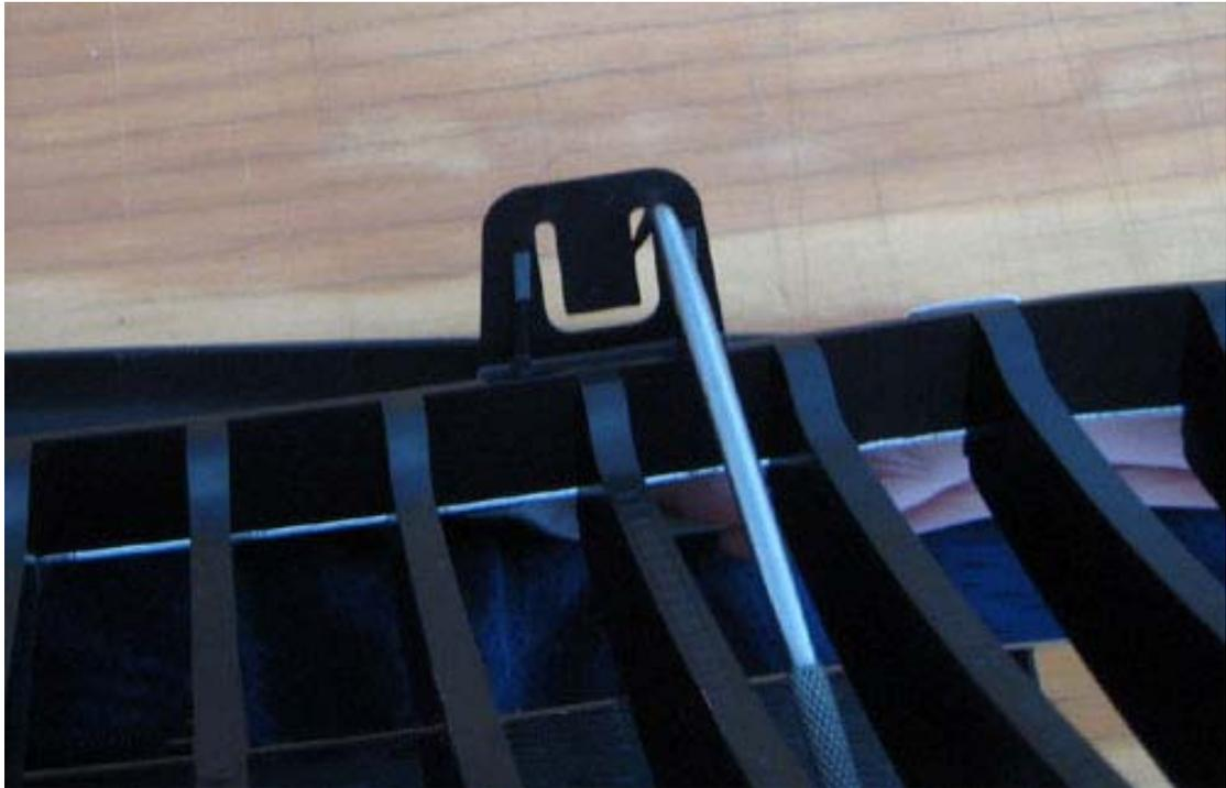
With the lower clips undocked, you can begin working on the upper clips. In order to access the clips, you want to pull up on the bumper trim and if you look in from the engine compartment, you will see the three clips. Use a flat blade screwdriver or the pointed end of the pick to push the clips down.
