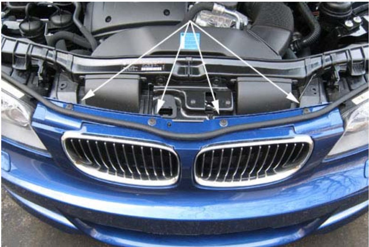
You will also want to lift the strip of insulation at the front of the hood off of it's sleeve. You remove it by pulling up.
