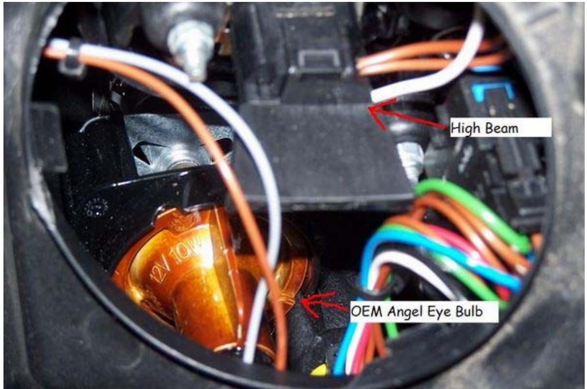
Step Seven: Custom Angel Eyes kept the same OEM seal to ensure the fitment back into the housing. The trick is there are 3 notches on the light housing, 2 are angled and one is not. The odd notch goes on top when inserted back into the Headlight and you are re-centering back into the Angel Eye hole. You can either plug in the new wiring harness before or after the re-insertion of the new Light.
