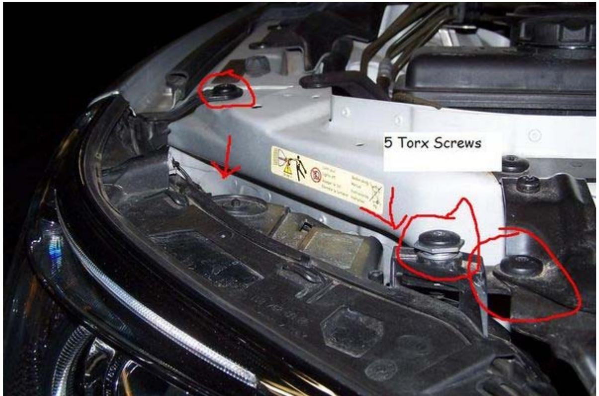
Step Four: Remove the back cover & gently push and wiggle your Headlight forward, your Headlight is now completely free to remove. You will have to gently wiggle it out, but it is pretty basic. (Important: twist off the Back Light cover, as it will catch when removing headlight).
