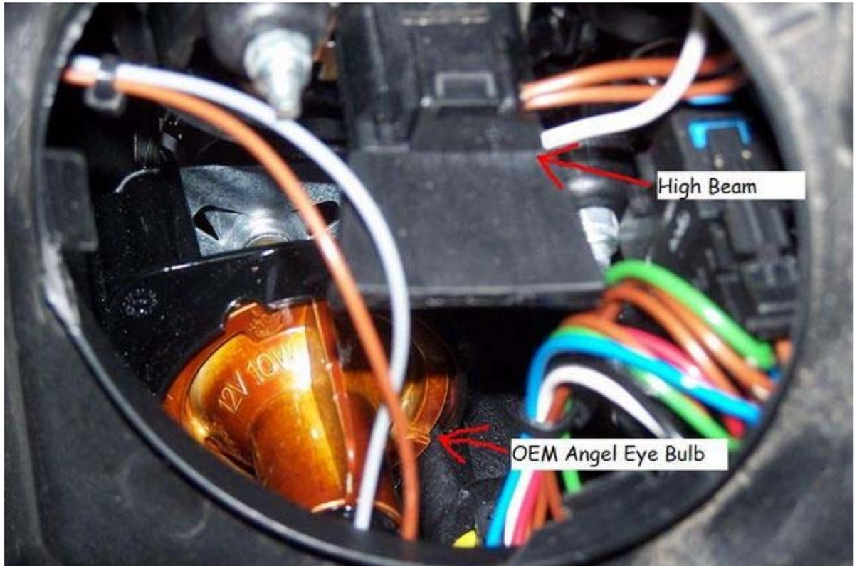
Step Two: Try and twist the bulb housing out by hand, if you succeed continue to step four, if not follow step three to remove it.
