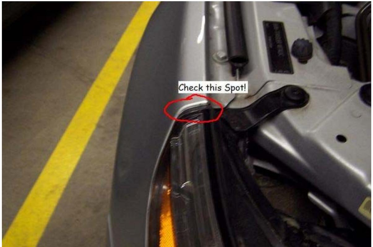
Step Two: Loosen and Remove the 3 top Screws (Do NOT drop screws down below the light, it may get lost or in a particularly difficult spot to retrieve).
