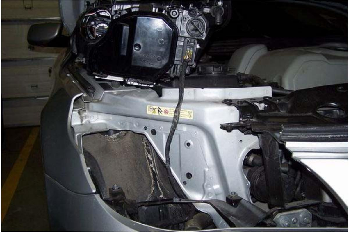
Step Six: If you look inside the headlight you will see it is a very tight workspace. This is the reason for removing the headlight; you will have more leverage this way. Twist out the High Beam bulb (quarter turn). Reach in and Gently Twist out the OEM Angel Eye Light Housing.
