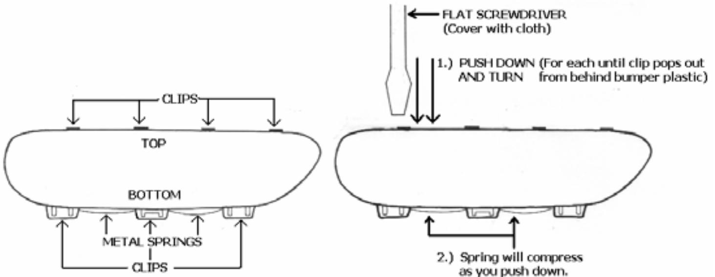
Take your painted reflector, and match up the shape of the reflector to the appropriate side (left and right reflectors are different), and install in the opposite way that you removed the original reflectors. Insert the bottom side of the reflector into the bumper and push down enough so that the springs at the bottom compress, then press the part against the car and it will snap into place.
