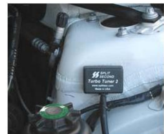
The internal adjustable boost setting.
