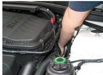
If the connection is done with the airbox in place, you have to work by feel.
