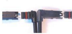
The Turbo Tuner 2 connectors plug in-line between the TMAP sensor and connector.
