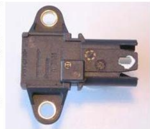
A clear view of the TMAP sensor.
