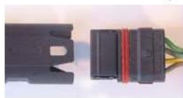
The connector separated from the TMAP sensor.
