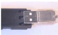
A USB connector makes a good removal tool.
